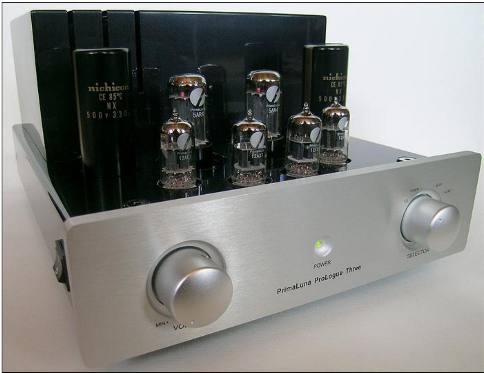
The chassis is heavy-gauge steel, fully vented at the bottom. Separate toroidal power transformers feed each channel's choke-regulated power supply for true dual-mono geometry. Parts goodies include Nichicon, Solen and Swelling capacitors; an Alps attenuator; ceramic tube sockets; and panel-mounted gold-plated connectors.
