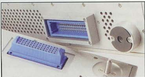
Power amp and PSU can only connect by stacking
